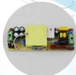
LED driver inside view
